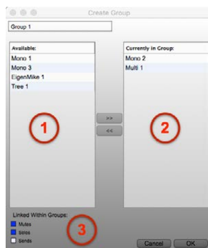
Figure 8. Creation/edition of a group. ① Available tracks. ② Tracks currently in group. ③ Group options.
