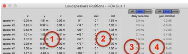
Figure 6. Configuration of the speaker layout for a panning bus. Speakers coordinates can be edited in Cartesian ① or spherical ② coordinates. The reproduction setup can be aligned in time ③ and level ④; delays and gains are automatically computed or manually entered.
