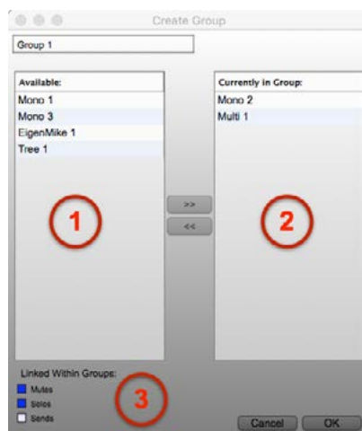
Figure 8. Creation/editing of a group. ① Available tracks. ② Tracks currently in group. ③ Group options.
