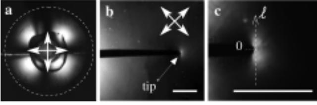
**Figure 3.** Birefringence signal for a double network with  $R = 0.5$ . (a) Snapshot taken before crack nucleation, while the oil is injected by the center of the cell. The dashed circle (true radius 8 cm) marks the boundary of the region occupied by the gel. (b) Crack propagating radially. (c) Zoom of the crack tip shown in (b). The scale of the white bars is 1.5 mm. The orientations of two crossed polarizers are indicated by the double arrows.
