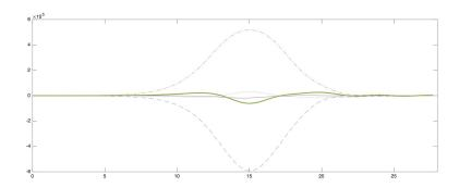
FIGURE 10. Decomposition of the vertical force  $F_{\text{vert}}$  (thick solid line) exerted on the structure, as in (74). Damping-excitation force  $F_{\text{D+E}}$  (dash-dot), restoring force  $F_{\text{restor}}$  (dash), force due to added mass  $F_{\text{added}}$  (dots) and nonlinear corrections  $F_{\text{NL}}$  (solid).
