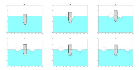
FIGURE 6. Return to equilibrium of a solid initially below its buoyancy line. Surface elevation (full), discharge (divided by a rescaling factor 5, dash), and initial condition (dots). The horizontal line on the structure marks the contact line at the equilibrium.
