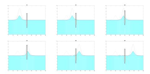
FIGURE 9. A solitary wave arriving on a freely floating structure (Boussinesq model). Surface elevation (full), initial condition (dots) and rescaled discharge (dash). The horizontal line on the structure marks the contact line at the equilibrium.
