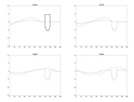
FIGURE 4. A wave arriving on a fixed floating structure. Surface elevation (full) and discharge (divided by a rescaling factor 5, dash).
