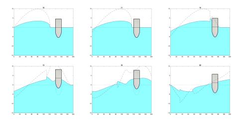
FIGURE 7. A wave arriving on a freely floating structure (nonlinear shallow water model). Surface elevation (full), initial condition (dots) and rescaled discharge (dash). The horizontal line on the structure marks the contact line at the equilibrium.
