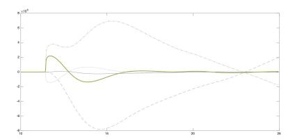
FIGURE 8. Decomposition of the vertical force  $F_{\rm vert}$  (thick solid line) exerted on the structure, as in (74). Damping-excitation force  $F_{\rm D+E}$  (dash-dot), restoring force  $F_{\rm restor}$  (dash), force due to added mass  $F_{\rm added}$  (dots) and nonlinear corrections  $F_{\rm NL}$  (solid).
