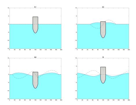
FIGURE 5. A solid in forced vertical motion. Surface elevation (full) and discharge (divided by a rescaling factor 5, dash), initial position (dots).
