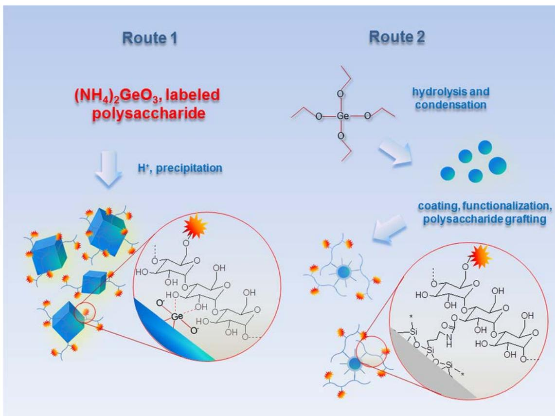
**Scheme 1** Formation of polysaccharide-coated GeO<sub>2</sub> nanoparticles
