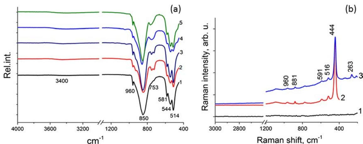
**Fig. 2** **a** FTIR spectra of GeO<sub>2</sub> nanoparticles: commercial powder (1), synthesized in water (2), synthesized in water solution of dextrin (3), synthesized in ethanol (4), and synthesized in ethanol and calcined at
