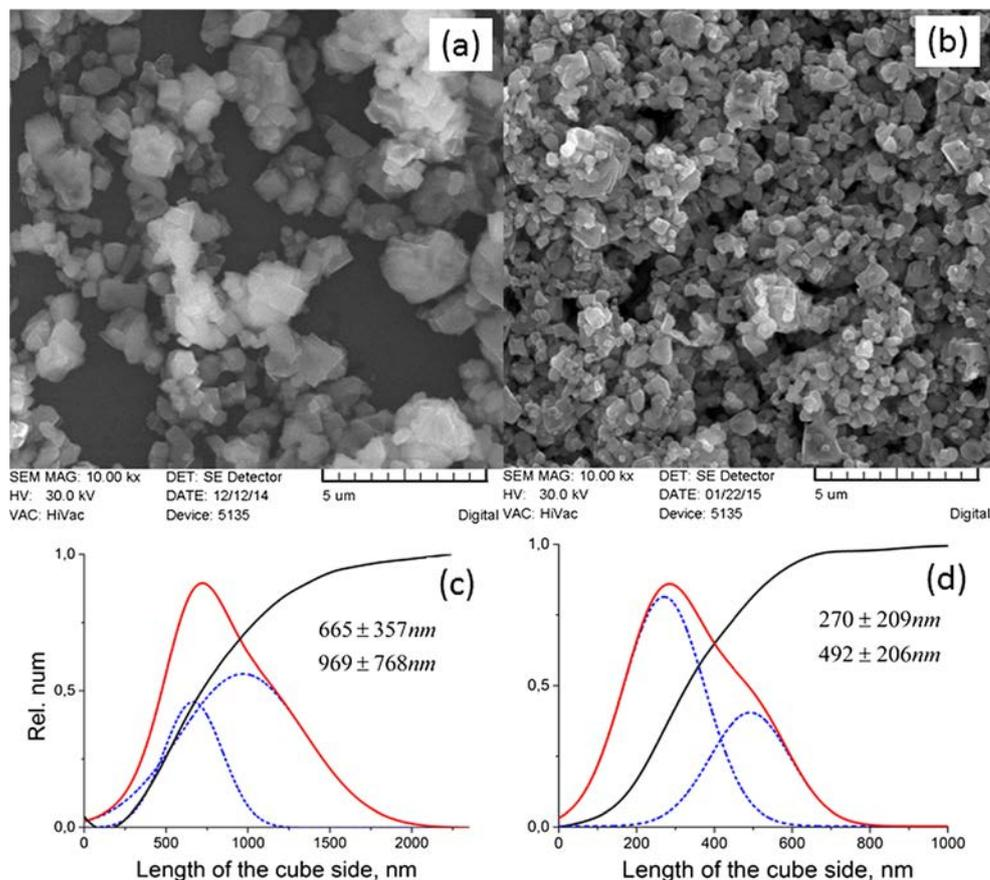
**Table 1** Properties of GeO<sub>2</sub> nanoparticles synthesized in water solutions containing polysaccharides
