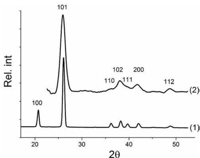
**Fig. 1** X-ray diffraction on GeO<sub>2</sub> nanoparticles: powder synthesized in a water solution (1) and dispersion in an ethanol reaction mixture (2)
