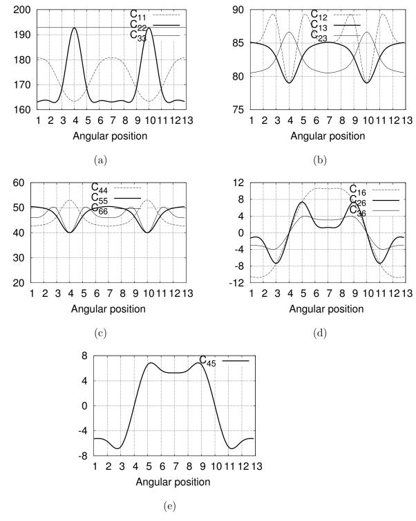
Figure 3: Variation of coefficients of the stiffness matrix (in GPa) from the  $1^{st}$  step of homogenization with respect to the angle  $\theta$  in inner layer.
