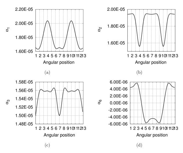
Figure 4: Variation of coefficients of the thermal expansion tensor (in  $\frac{1}{K}$ ) from the 1<sup>st</sup> step of homogenization in inner layer: (a)  $\alpha_1$ , (b)  $\alpha_2$ , (c)  $\alpha_3$  and (d)  $\alpha_6$ . In addition  $\alpha_4 = \alpha_5 = 0$ .
