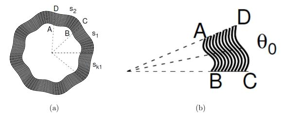
Figure 2: (a) Cross section of the tube divided into  $k_1$  sectors and (b) a typical sector.
