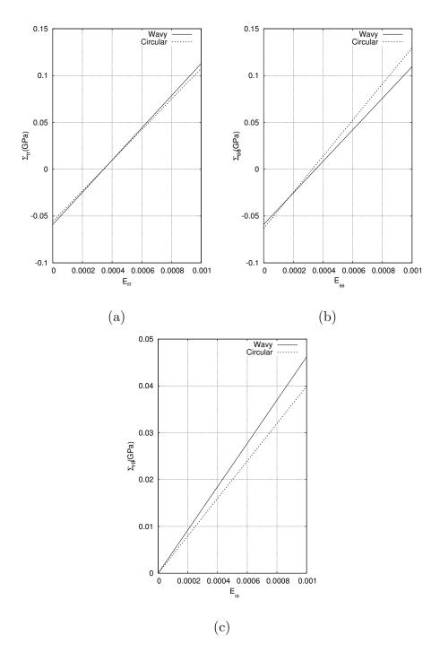
Figure 6: (a) Effective radial stress vs effective radial strain, (b) effective hoop stress vs effective angular strain and (c) effective shear (in the cross section) stress vs effective shear strain, for  $\Delta T$ =10 K in inner layer.
