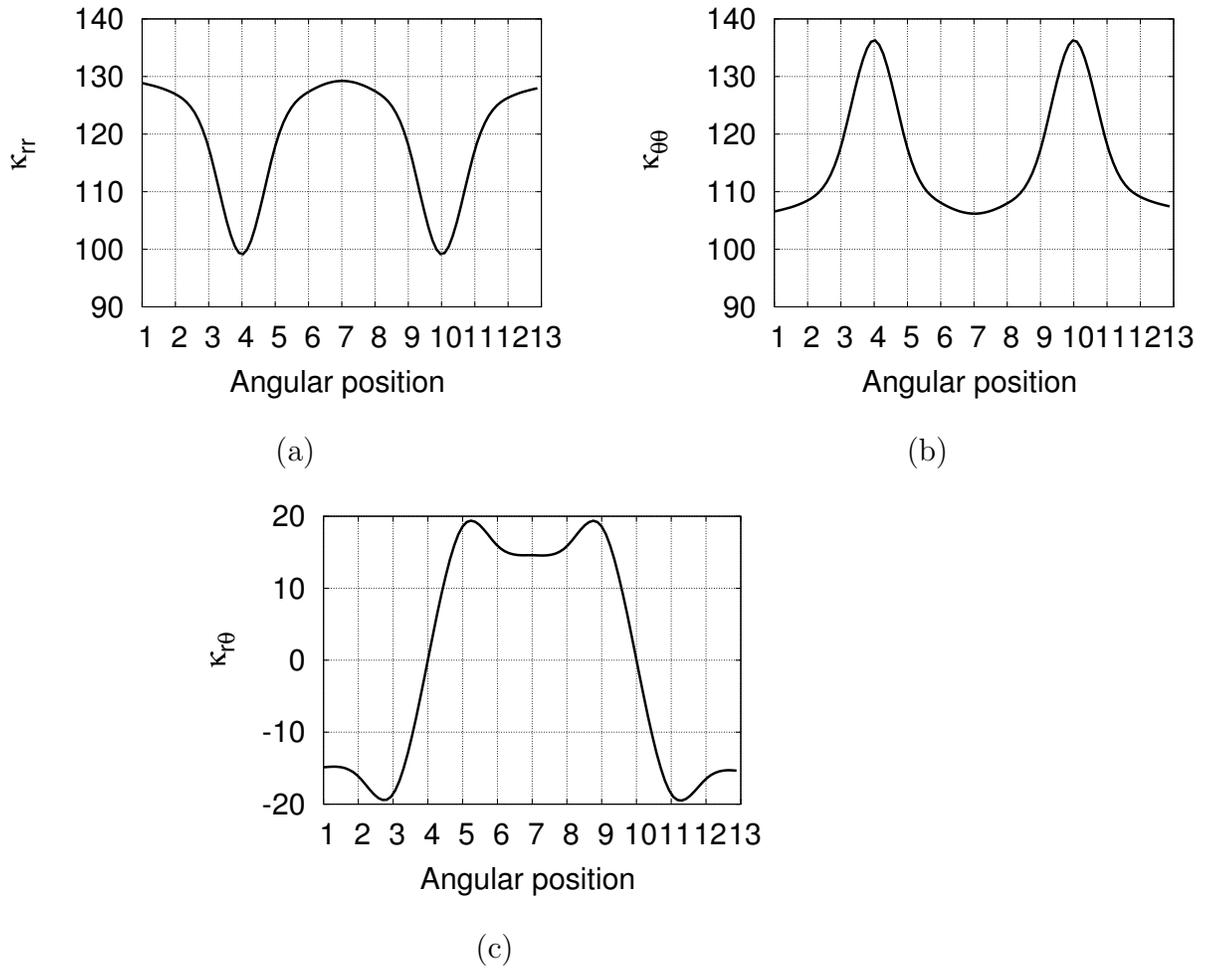
Figure 5: Variation of coefficients of the thermal conductivity tensor (in  $\frac{W}{mK}$ ) from the 1<sup>st</sup> step of homogenization in inner layer: (a)  $\kappa_{rr}$ , (b)  $\kappa_{\theta\theta}$  and (c)  $\kappa_{r\theta}$ . In addition  $\kappa_{zz}=136.302 \frac{W}{mK}$  and  $\kappa_{rz}=\kappa_{\theta z}=0$ .
