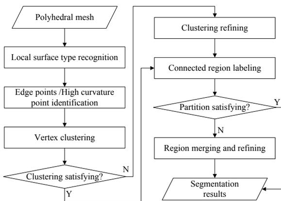
Figure 3. Shape segmentation process.
