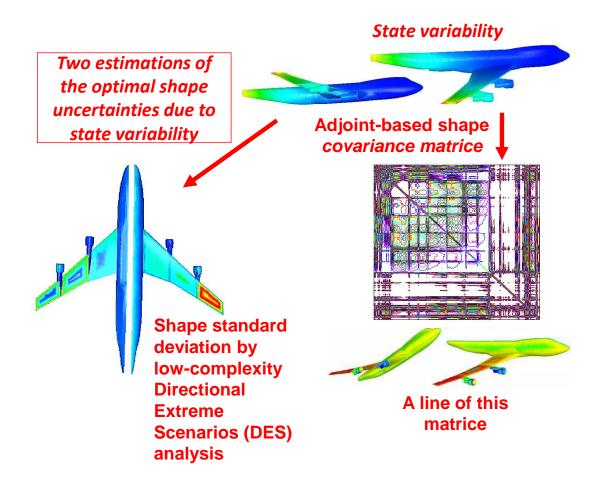
**Fig. 6** Two approaches to build  $diag(Cov_x)$  from  $diag(Cov_{u^*})$  indicating the variability of  $\mathbf{u}^*$  over the shape. The covariance distribution over the shape of the aircraft shows that for the design to be robust in variable flight conditions the engines pylon, fairing and air intakes should have different shapes following their position on the wing.
