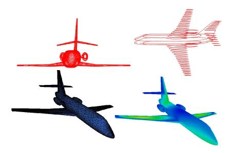
Fig. 4 CAD-free shape parameterization (lower-left) and by-section definitions (upper) of the shape for geometric constraints enforcement. Lower-right is one single  $\nabla_{\mathbf{x}}C_d - \langle \nabla_{\mathbf{x}}C_d, \pi \rangle \pi$  described in section 9.1.3 for this CAD-free parameterization.
