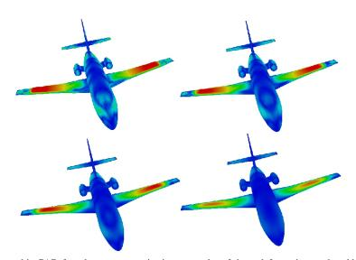
Fig. 5 Regularity control in CAD-free shape parameterization: examples of shape deformation produced by our optimization procedure for different regularity requirements.
