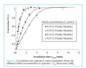
Aillet et al (5-6) have proposed a simple modelling approach to describe the coupling between photochemical kinetics, mass, momentum and radiative transfer equations inside flow photoreactors. Assuming a plug-flow behaviour, this model allows predicting the conversion X at the photoreactor outlet with the irradiation time, according to:
