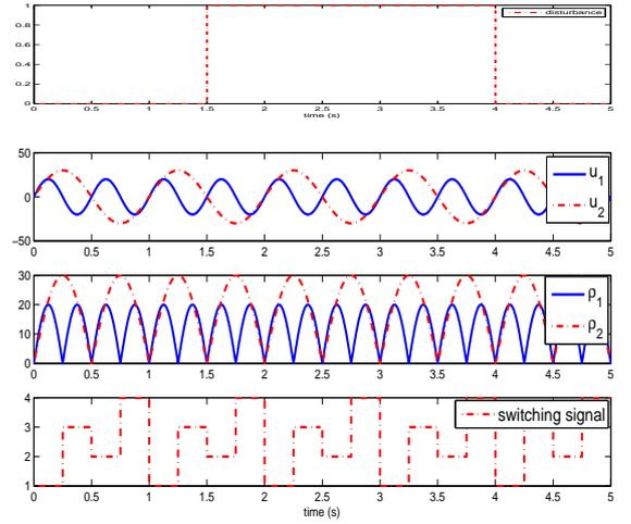
Fig. 8. Disturbance, control inputs, varying parameters, switching signal
