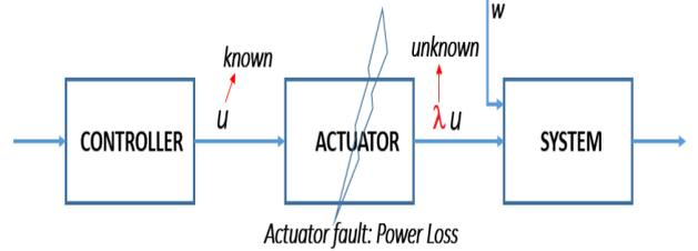
Fig. 1. System with actuator fault
