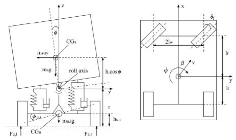
Fig. 1 Yaw-Roll model of single unit heavy vehicle [5].
