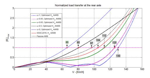
Figure. 10 Effect of the forward velocity on the normalized load transfer: rear axle R<sub>r</sub>.
