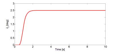
Figure. 7 Steering angle  $\delta_f$  during cornering maneuver.
