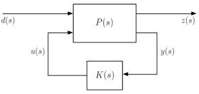
Fig. 2 Generalized control structure.
