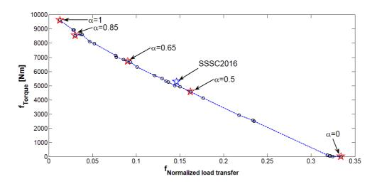
Figure. 4 The optimization results of some points in the Pareto frontier for the active anti-roll bar on heavy vehicle.
