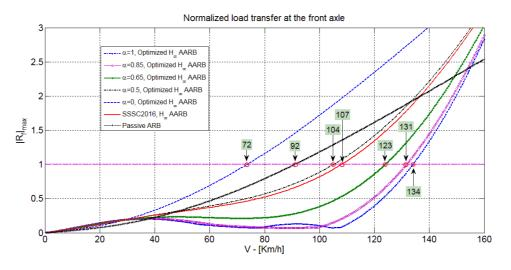
Figure. 9 Effect of the forward velocity on the normalized load transfer: front axle R<sub>f</sub>.
