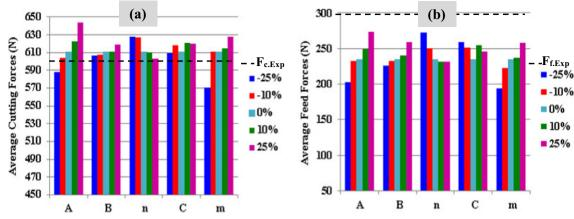
Fig. 14 Parametric study of the JC plastic model effect on cutting and feed forces ( $V_c = 75 \text{ m/min}, a_p = 3 \text{ mm}, \text{ and } f = 0.1 \text{ mm/rev}$ )
