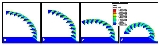
Fig. 17 Chip morphology dependency to damage evolution definition ( $\mathbf{a} - 25\% G_{f0}$ ,  $\mathbf{b} - 10\% G_{f0}$ ,  $\mathbf{c} + 10\% G_{f0}$ , and  $\mathbf{d} + 25\% G_{f0}$ )
