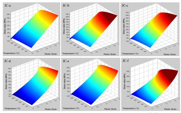
Fig. 2 Flow stress evolution with the temperature and the strain rate corresponding to different plastic JC sets ( $\dot{\varepsilon} = 10^4 \text{ s}^{-1}$ )
