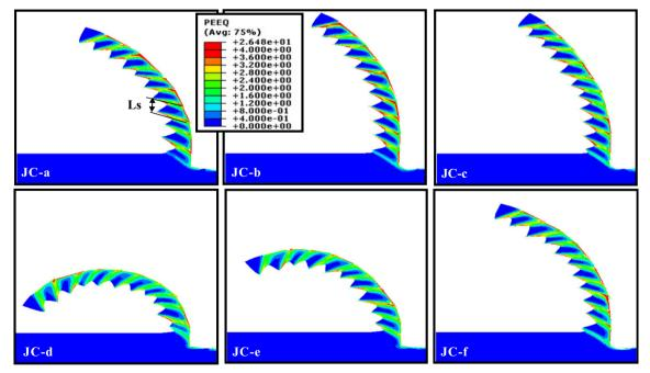
Fig. 3 Chip morphology and strain evolution dependency to JC plastic parameters ( $V_c = 75 \text{ m/min}, a_p = 3 \text{ mm}, \text{ and } f = 0.1 \text{ mm/rev}$ )
