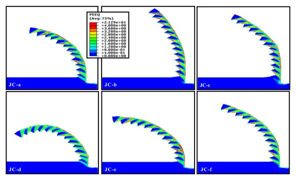
Fig. 4 Dependency of the chip morphology and the equivalent plastic strain evolution to JC plastic coefficients ( $V_c = 180 \text{ m/min}$ ,  $a_p = 3 \text{ mm}$ , and f = 0.1 mm/rev)
