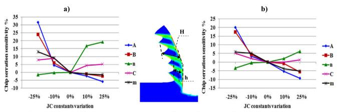
Fig. 10 Chip segmentation sensitivity factor dependency to JC plastic coefficients definition under different cutting speeds (a  $V_c = 75$  m/min and b  $V_c = 180$  m/min)
