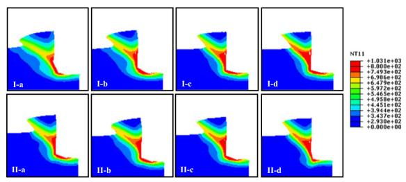
Fig. 11 Temperature evaluation within the primary shear zone under different value of A (I) and B (II) (a - 25, b - 10, c + 10, and d + 25 %)
