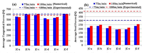
Fig. 7 Dependency of the average cutting (a) and feed (b) forces to JC plastic parameters with respect to the cutting speed
