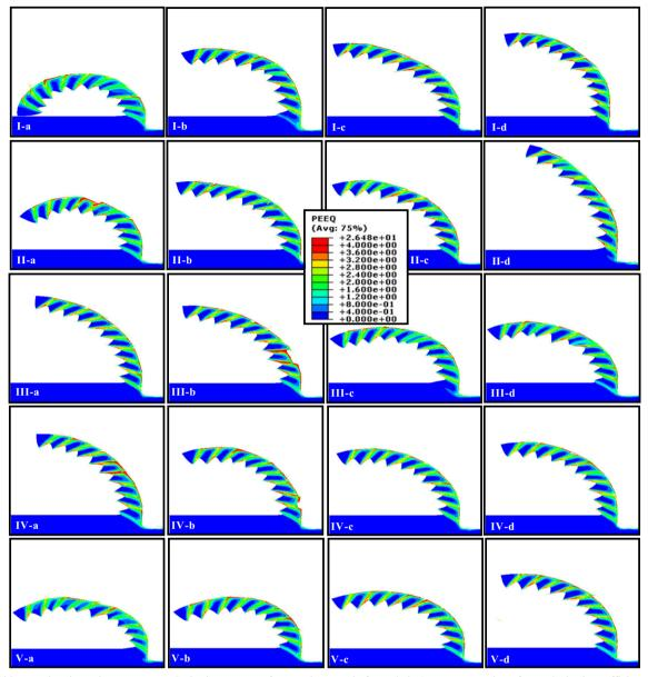
**Fig. 8** Chip sertation dependency to every JC plastic parameter for a cutting speed of 75 m/min (*I*, *II*, *III*, *IV*, and *V* refer to JC plastic coefficients (*A*, *B*, *n*, *C*, and *m*, respectively) while *a*, *b*, *c*, and *d* correspond to the range of their variations (-25, -10, +10, and +25 %, respectively))
