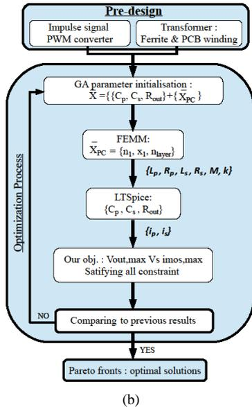
Fig.3 (a) Synopsis and schematic of the impulse transmission function based on a magnetic transformer. (b) GA flowchart for overall system optimization based on FEMM<sup>TM</sup> and LTSpice<sup>TM</sup>.
