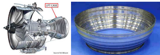
Fig.1 Turbine casing work-piece
