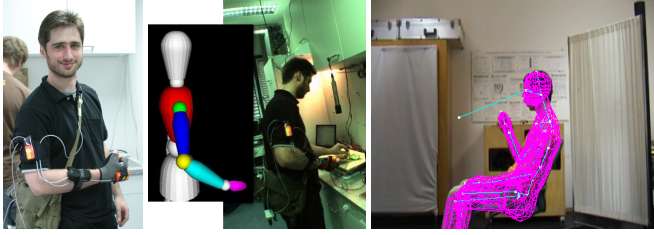
Fig.6: Sensing, reaching, and grasping activities using tiny inertial measurement units (left). Estimating the pose of people by accurately matching digital human models into image sequences (right).
