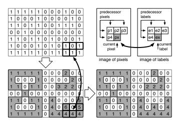
Fig. 1 An example of 8-connected component labeling with Rosenfeld algorithm. Top: binary image, bottom left: image of temporary labels, bottom right: image of final labels
