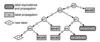
**Fig. 5** 8-connected Decision Tree for a 4-pixel mask. Label equivalence and the propagation to  $e_x$  in dark gray
