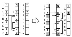
**Fig. 6** Suzuki tables: Root, Next and Tail before connecting x=1 and y=2.  $S1=\{1,3,7\},\ S2=\{2,6,4\}$  and after connecting  $S1=\{1,3,7,2,6,4\}$ . Modified Data are in gray.
