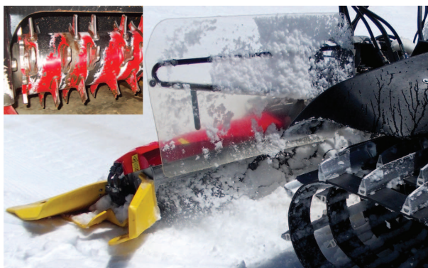
FIGURE 3: The tiller is mounted at the rear of a grooming machine and consists of a high speed rotating shaft (cutter bar) with multiple tines which acts as a mixer for the top of the snowpack
