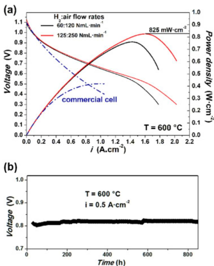
Fig. 7. (a)  $i$ - $V$  and power density curves of a single cell with  $\text{Pr}_6\text{O}_{11}$  infiltrated cathode, measured at  $600 \text{ }^\circ\text{C}$ , for two different gas flow rates; (b) Cell voltage measured at  $600 \text{ }^\circ\text{C}$  and  $0.5 \text{ A}\cdot\text{cm}^{-2}$  for 840 h. The characteristics of a commercial cell from Elcogen have been measured in a ( $\text{H}_2$ :air) flow rate =  $60:120 \text{ NmL}\cdot\text{min}^{-1}$ .
