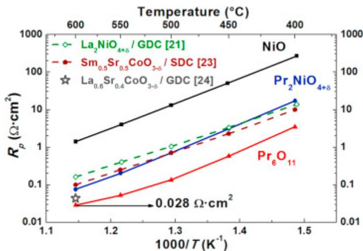
Fig. 4. Arrhenius plots of the polarization resistance of Gd-doped ceria backbones infiltrated with  $\text{Pr}_6\text{O}_{11}$ , compared with results for electrodes infiltrated with NiO and  $\text{Pr}_2\text{NiO}_{4+\delta}$ , and reported results for  $\text{La}_2\text{NiO}_{4+\delta}$  infiltrated into GDC [22],  $\text{Sm}_{0.5}\text{Sr}_{0.5}\text{CoO}_{3-\delta}$  infiltrated into SDC [23], and  $\text{La}_{0.6}\text{Sr}_{0.4}\text{CoO}_{3-\delta}$  infiltrated into GDC [24].
