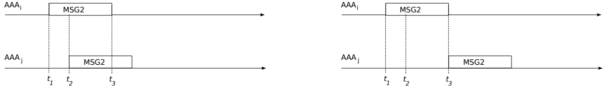
Figure 3.3: On the left-hand side: actions execution in the real case. On the right-hand side: actions execution in NS simulations
