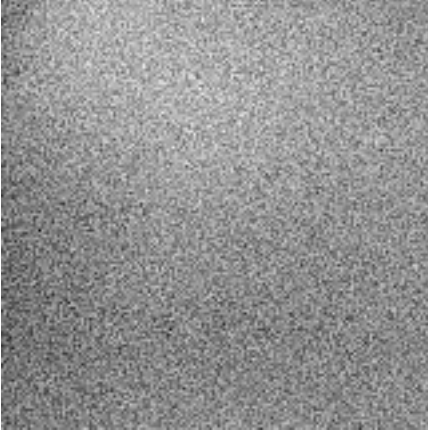
Figure 2. Illustration of the sensor noise n on a picture at 2000 ISO captured with the Leica Monochrome camera. Inactivate the interpolation process of your pdf viewer for correct rendering. The pixel amplitudes are scaled for visualization purposes.
