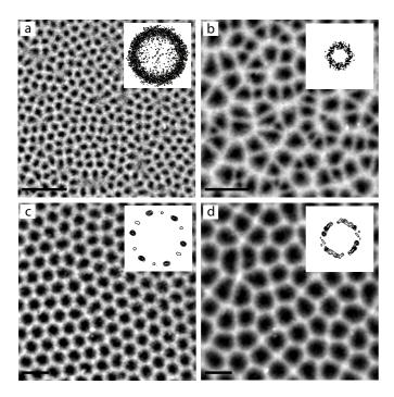
Fig. 3: Typical evaporation-driven BM patterns (H = 3 cm): (a) HFE-7000,  $\epsilon = 0.2$ ; (b) HFE-7000,  $\epsilon = 2$ ; (c) HFE-7300,  $\epsilon = 0.2$ ; (d) HFE-7300,  $\epsilon = 2$ . White bars are 4 mm long. Topright insets: contour lines of power (Fourier) spectrum.
