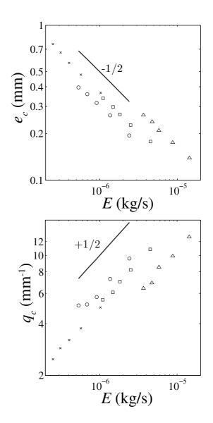
Fig. 1: Measured critical liquid thickness  $e_c$  (top) and critical wave number  $q_c$  (bottom) as a function of the evaporation rate E, for different liquids (triangles: HFE-7000; squares: HFE-7100; circles: HFE-7200; crosses: HFE-7300). Straight lines indicate the theoretical scaling laws (see text).
