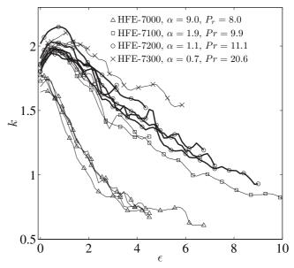
Fig. 4: Measured dimensionless wave number k vs. supercriticality  $\epsilon = (Ma - Ma_c)/Ma_c$ . For each liquid, evolutions corresponding to all five container heights are represented. Pr is the Prandtl number of the liquids.
