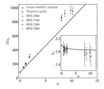
Fig. 2: Measured critical Marangoni numbers (symbols) as a function of  $\alpha$ , for the four different liquids and the five container heights. Inset: corresponding measured critical wave numbers. Theoretical laws are shown as plain curves.
