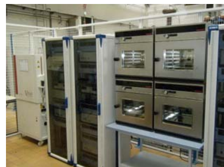
Figure 2. Experimental bench for lifetime measurement under PWM stress.
