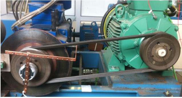
Fig. 1. Experimental test bench composed of an 30-kW IM (right), a belt-pulley transmission system (middle) and a direct-current machine (left).
