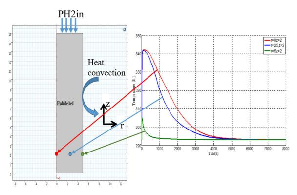
Fig 5: Bed temperature vs. time for various positions in the reactor
