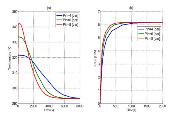
Fig 6: Effect of the supply pressure
