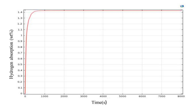
Fig 4: Concentration vs. time during hydrogen absorption
