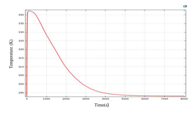
Fig 2: Bed temperature vs. time during absorption
