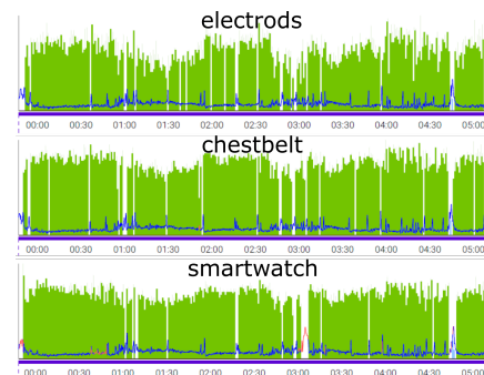
Figure 1: HR (blue line) and HRV (green area) from electrodes, chestbelt and smartwatch wear during the same night.
