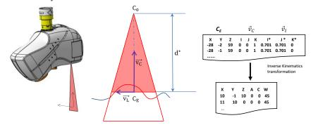
Fig. 2. Parameters defining the sensor trajectory for on-machine inspection
