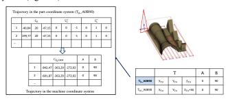
**Fig. 6.** Scanning trajectories for test (A =  $0^{\circ}$ ; B =  $90^{\circ}$ , z= 0 mm).
