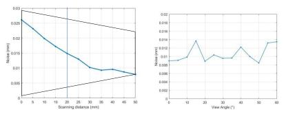
Fig. 5. Noise in function of the scanning distance (a) and the view angle (b).
