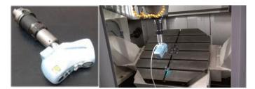
Fig. 1. Laser-sensor in the machine-tool
