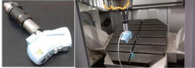
**Fig. 1.** Laser-sensor in the machine-tool
