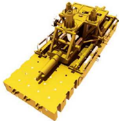
Figure 1. PLET with a fixed skirted mudmat and a railing system to accommodate the expansion (Wallerand et al., 2015).
