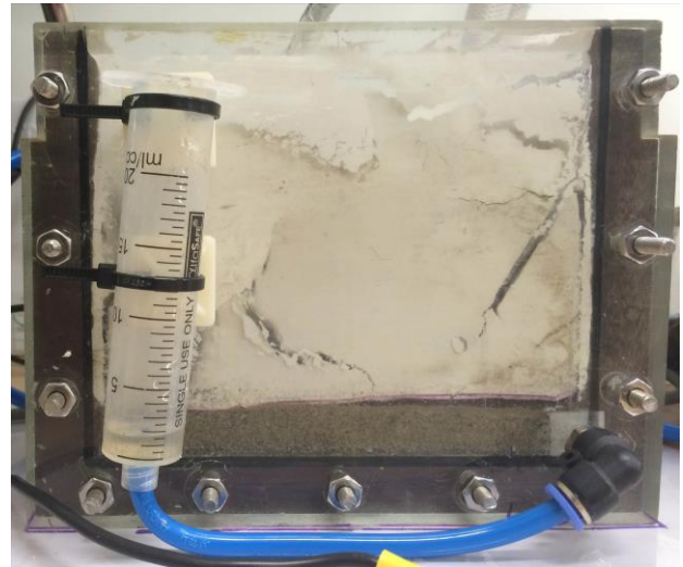
Figure 8. Crack formation. Test T1.
