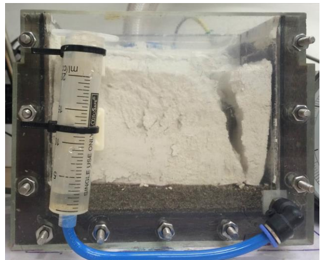
Figure 9. Crack formation. Test T2.
