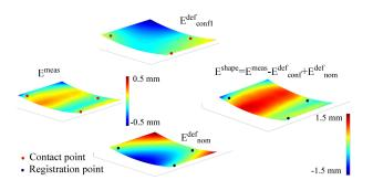
FIGURE 8: Evaluation of the shape deviation field
