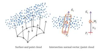
FIGURE 3: Evaluation of the local geometrical deviation
