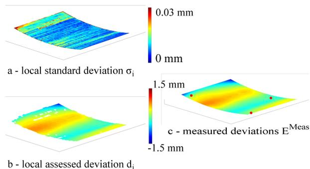
FIGURE 7: Evaluation of the measured deviation field,  $E^{\text{meas}}$
