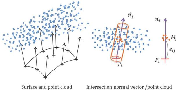
FIGURE 3: Evaluation of the local geometrical deviation
