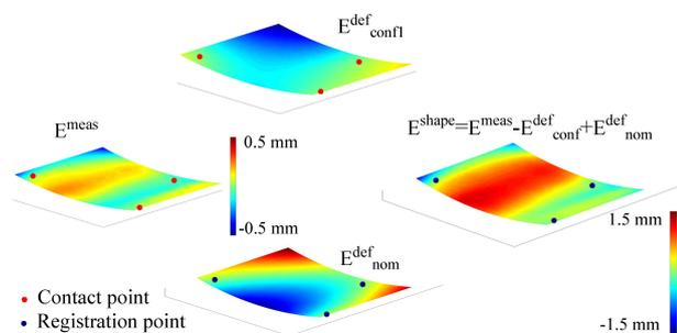
FIGURE 8: Evaluation of the shape deviation field
