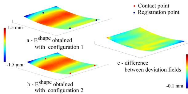
FIGURE 9: Difference between deviation fields considering 2 measurement configurations
