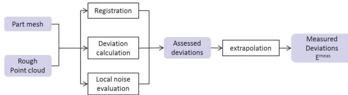
FIGURE 4: From measured points to measured deviations
