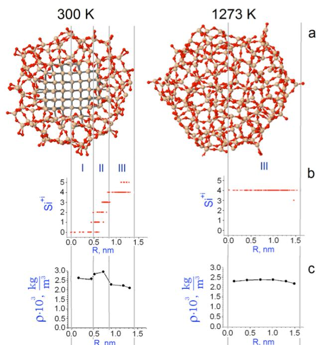
**Figure 2** - Analysis of (a) post-oxidation Si-structures obtained at 300 K and 1273 K by (b) their Si-suboxide components and (c) their mass density distribution. Reproduced from [89] with permission from the American Chemical Society.
