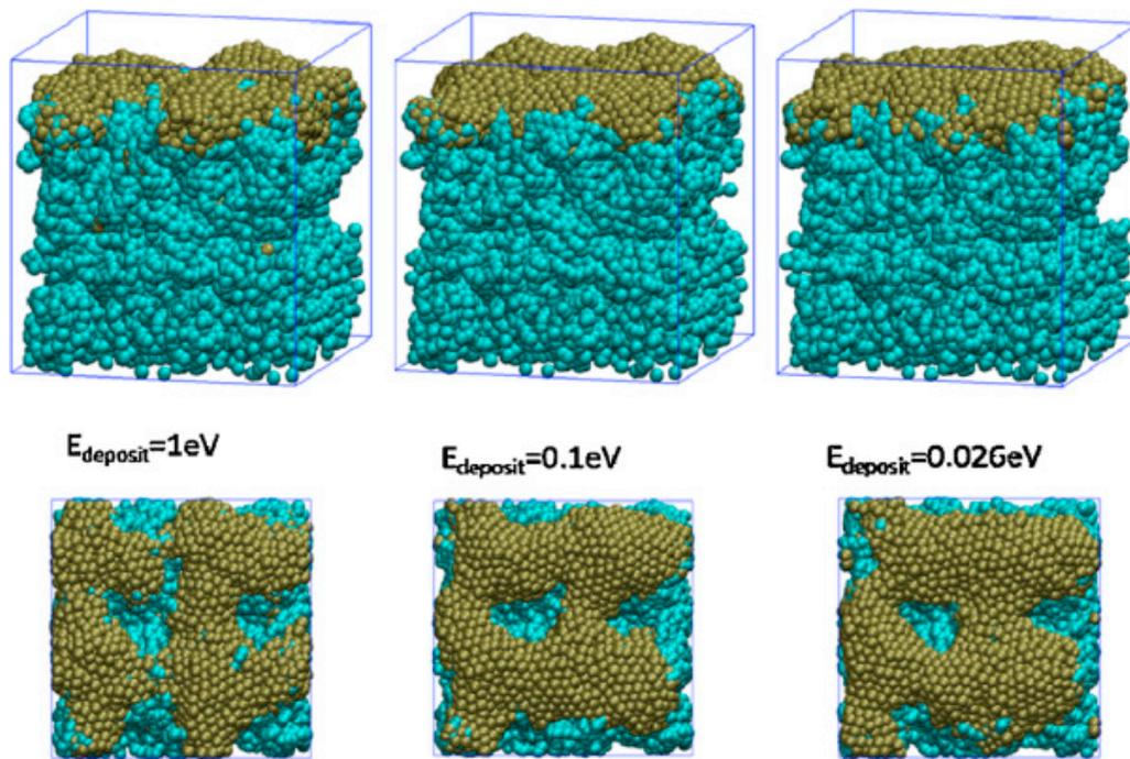
**Figure 1** - Snapshots of Pt deposition on the porous carbon substrate. The green spheres represent C-atoms and the brownish spheres represent Pt-atoms. Reproduced from [60] with permission from Elsevier.
