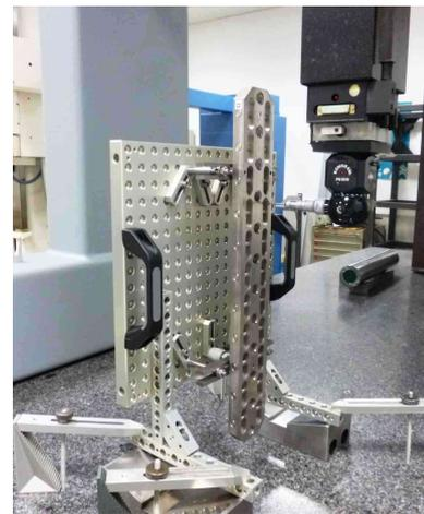
Figure 8. MFB calibration set-up on CMM at LNE.
