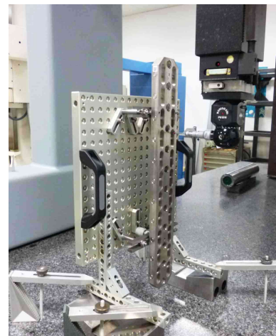
Figure 8. MFB calibration set-up on CMM at LNE.
