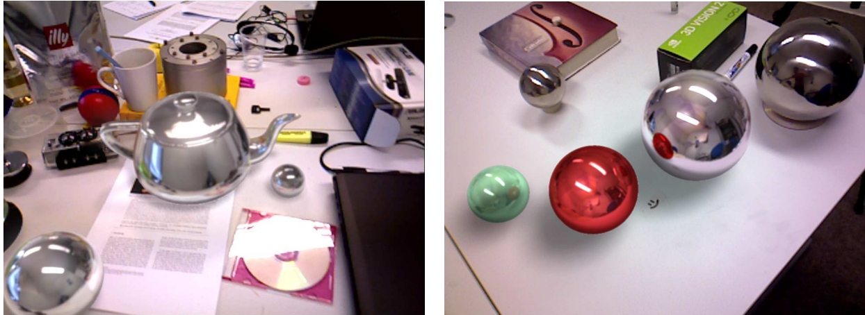
Figure 1: Realistic HDR reflections on several virtual objects with shadow casting, rendered in real-time from live video stream. The reflection maps have been computed from a dense live reconstruction of the scene's light-field.
