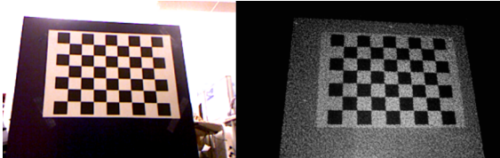
Figure 2: RGB and IR images of the calibration pattern.
