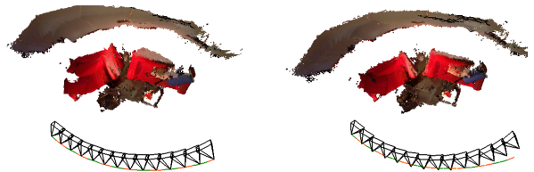
Figure 11: The effect of sparse bundle adjustment illustrated. Minor error at the end of the trajectory is corrected in the right side image. The dense scene geometry becomes precise with correct poses. Notice especially the sofa shape before and after the correction.
