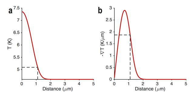
Extended data Figure 2 : Temperature profile in the niobium film under laser heating.
