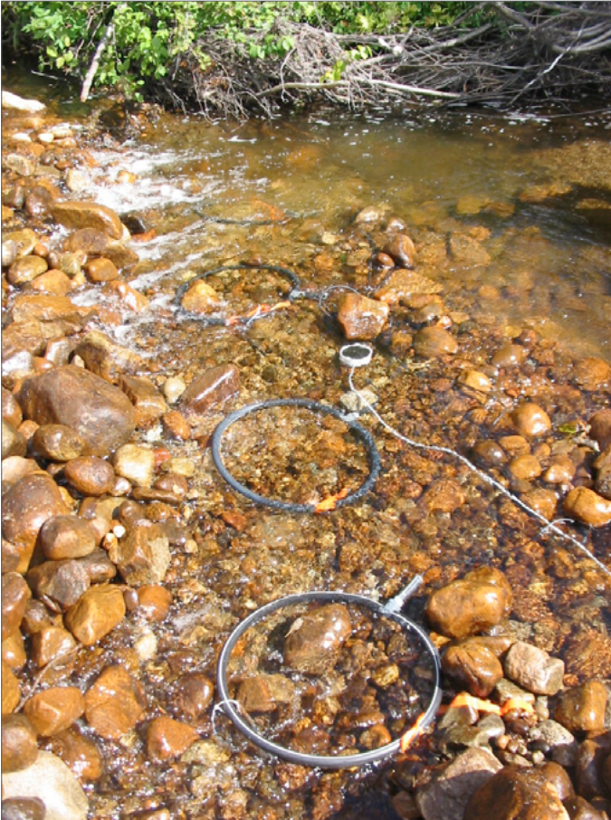
Figure 2. Antennae before they are covered with stream substrate
