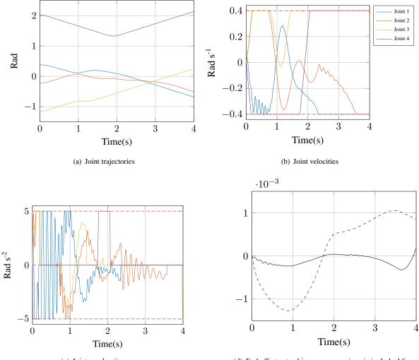
(d) End-effector tracking error: error in x is in dashed line and in y in solid line
