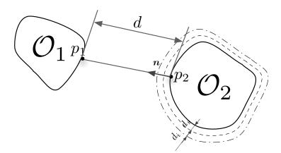
Figure A1. Collision avoidance as kinematics inequality constraints
