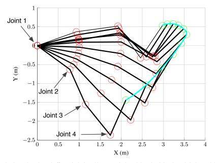
Figure 1. Planar redundant robot: the end-effector is designed by green circle and the robot joints by red circles, and the end-effector trajectory by solid cyan line.
