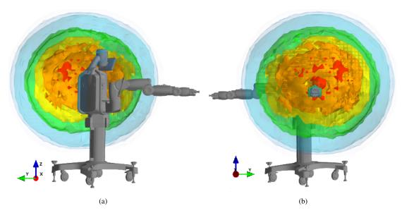
Figure 4. 6D Kinematic reachability space of Baxter's left arm. The color density increases according to the number of possible configurations.
