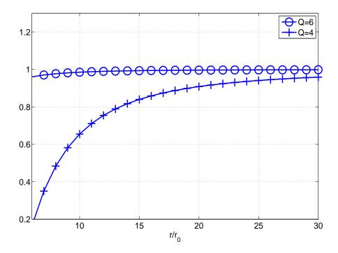
Fig.9 Ratio of the approximate CRB(r) to the exact one for uniform square-based arrays.
