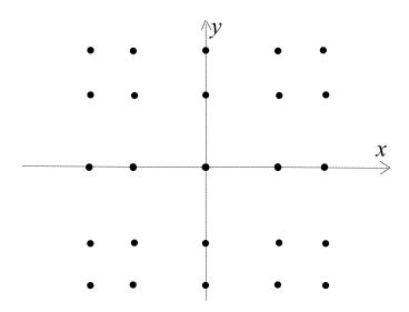
Fig.3 Square-based centro-symmetric array.
