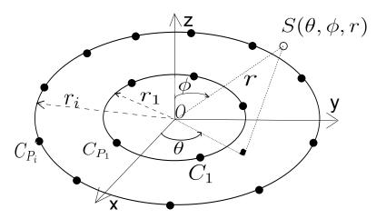
Fig.1 Concentric uniform circular-based array and source parameters.
