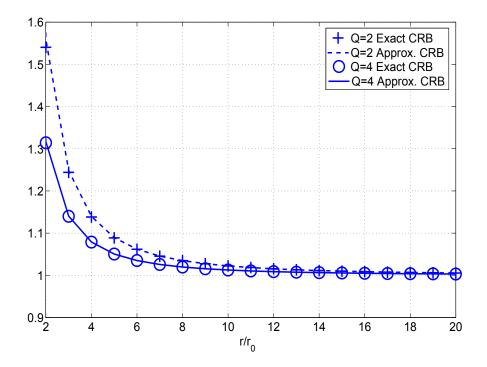
Fig.7 Approximate and exact ratios  $CRB(\theta)/CRB_{FF}(\theta)$  for uniform square-based arrays.
