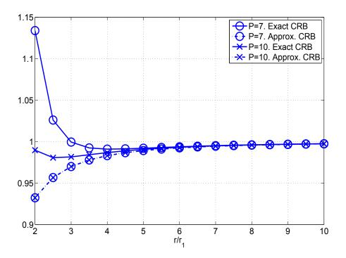
Fig.5 Approximate and exact ratios  $CRB(\phi)/CRB_{FF}(\phi)$  for the UCA.
