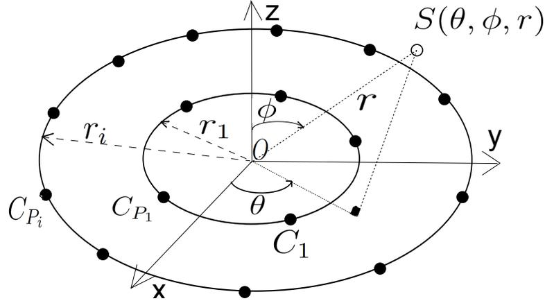
Fig.1 Concentric uniform circular-based array and source parameters.
