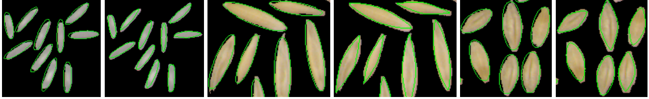
Figure 1. Fitting results on isolated grain kernels to illustrate the interest of superellipse (even) against ellipse (odd).
