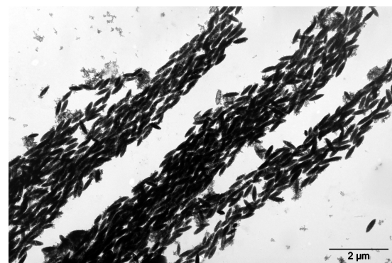
Figure 4. TEM image of iron nanoparticles coated with silica dried in the presence of a magnetic field H=120\text{kA/m}
