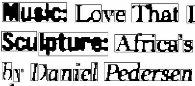
Fig. 4 Illustration of broken and damaged characters in a low resolution document image.
