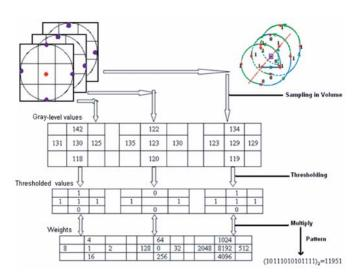
Fig. 8. Procedure of VLBP<sub>1,4,1</sub> [60].
