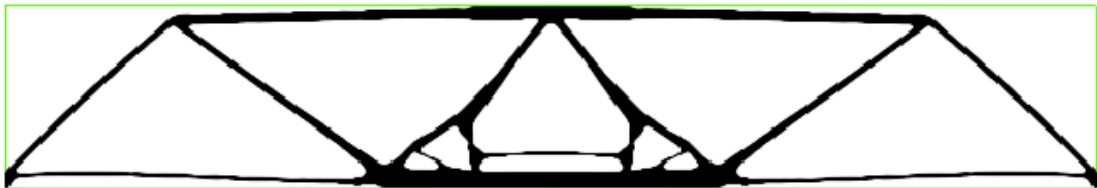
Figure 3: Optimized shape \Omega^{opt} for (73) with \alpha = 0.3 and C = 2\xi M .
