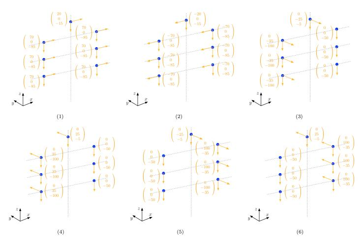
Figure 23. Definition of the six load cases considered in the pylon design example of Section 6.4
