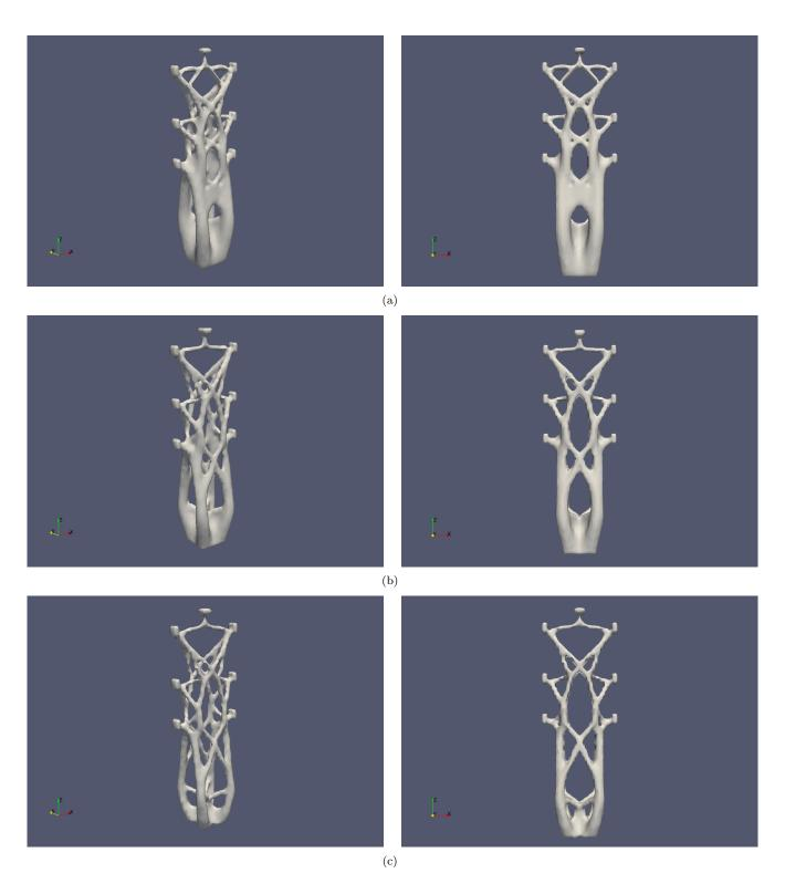
FIGURE 29. Optimized designs in the minimization of  $S(\Omega)$  performed in Section 6.4.3 with target volumes (a)  $V_T = 0.1|D|$ ; (b)  $V_T = 0.075|D|$ ; (c)  $V_T = 0.05|D|$ .
