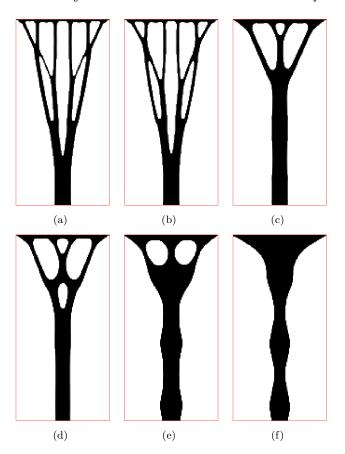
FIGURE 14. Optimized shapes for problem (28) setting: (a) t = 1.0; (b) t = 0.90; (c) t = 0.60; (d) t = 0.45; (e) t = 0.35; (f) t = 0.15;.
