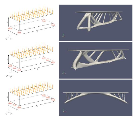
FIGURE 2. Three optimized designs of a three-dimensional bridge associated to different sets of fixations (see [12] for details).
