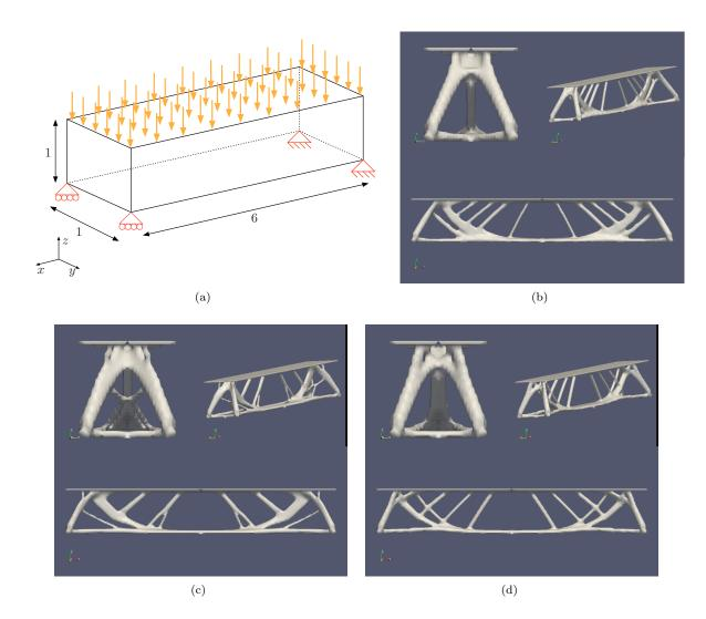
FIGURE 15. (a) Description of the optimal bridge test case; (b) optimized shape without adding any thickness constraints; (bottom) optimized shapes for problem (31) setting: (c)  $m_1 = 0.1$ ; (d)  $m_1 = 0.01$ .
