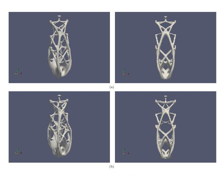
FIGURE 30. Optimized design in the minimization of  $S(\Omega)$  under a volume constraint  $V_T = 0.1|D|$ , and anisotropic maximum thickness constraints associated to the parameter (a)  $\delta = 4\sqrt{\min\{m_1, m_2, m_3\}}\Delta x$ ; (b)  $\delta = 3\sqrt{\min\{m_1, m_2, m_3\}}\Delta x$  (Section 6.4.3).
