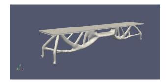
FIGURE 7. (Left) Reproduction of the definition of the test-case of Figure 2 modified by the addition of an 'empty' non-optimizable zone; (right) resulting optimal shape.
