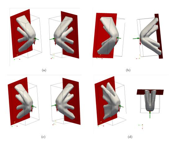
FIGURE 17. Optimized shapes for the short cantilever test case with different metric tensors M in the definition of the anisotropic maximum thickness (a)  $m_1 = 0.01$ ; (b)  $m_1 = 0.01, m_2 = 0.01$ ; (c) one constraint with  $m_1 = 0.01, m_2 = 1.0$  and a second constraint with  $m_1 = 1.0, m_2 = 0.01$ ; (d)  $m_3 = 0.01$ .
