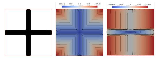
FIGURE 6. (Left) One shape  $\Omega$  (in black); (middle) isolines of the isotropic distance function  $d_{\Omega}$ ; (right) isolines of the anisotropic distance function  $d_{\Omega}^{M}$  associated to the tensor (14).
