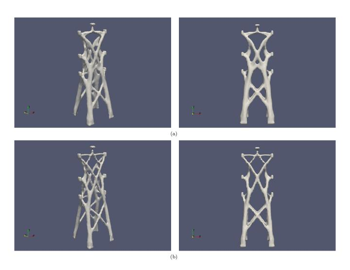
FIGURE 25. Optimized designs for the minimization of  $S(\Omega)$  with target volumes (a)  $V_T = 0.075|D|$  and (b)  $V_T = 0.05|D|$ .
