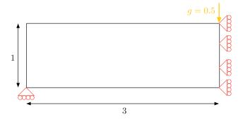
FIGURE 18. Setting of the MBB beam example of Section 6.3.3.
