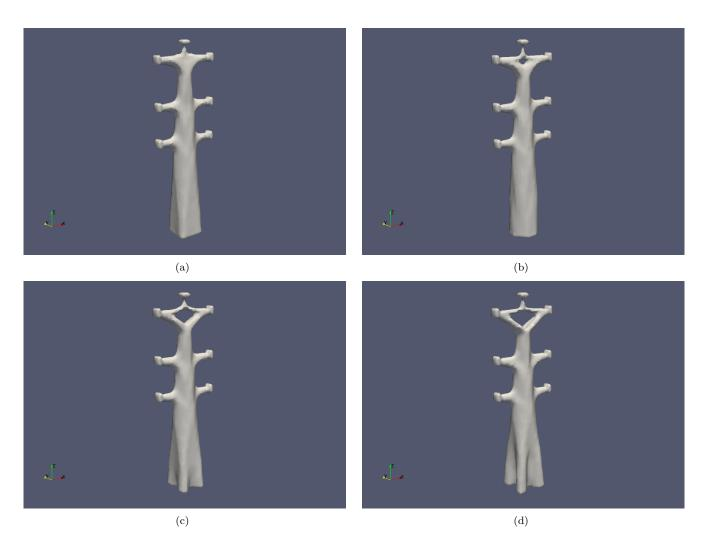
FIGURE 28. Optimized designs under the constraint that the shape resembles the design  $\Omega_T$  of Figure 27 (Section 6.4.2); values of the weighting coefficient (a) t = 0.2; (b) t = 0.3; (c) t = 0.4; (d) t = 0.6.
