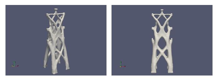
Figure 24. Resulting pylon from the minimization of  $S(\Omega)$  with target volume  $V_T = 0.1|D|$ .
