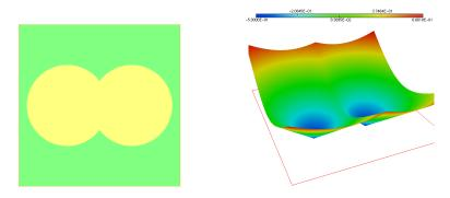
FIGURE 4. (Left) One shape  $\Omega \subset \mathbb{R}^2$ , and (right) the graph of an associated level set function.
