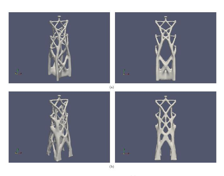
FIGURE 26. Optimized design in the minimization of  $S(\Omega)$  under a volume constraint  $V_T = 0.1|D|$ , and anisotropic maximum thickness constraints associated to the parameter (a)  $\delta = 4\sqrt{\min\{m_1, m_2, m_3\}}\Delta x$ ; (b)  $\delta = 3\sqrt{\min\{m_1, m_2, m_3\}}\Delta x$  (Section 6.4.1).
