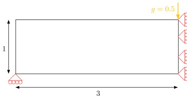
FIGURE 18. *Setting of the MBB beam example of Section 6.3.3.*
