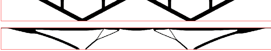
FIGURE 10. (Top) ‘target’ domain \Omega_T provided by the designer; (bottom) optimized shape for the problem (27) starting from \Omega_T .
