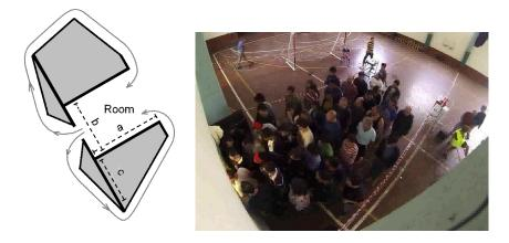
Figure 1: (Left) Sketch of the experimental geometry, with  $a=7.3\,\mathrm{m},\,b=3.5\,\mathrm{m},\,\mathrm{and}\,\,c=4.3\,\mathrm{m}.$  (Right) snapshot of an evacuation.
